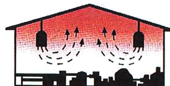
CONVECTION HEAT Forced air convection heat works from the top down, heating the air first and stratifying from the ceiling downward. More heat is wasted in the upper area the building.
