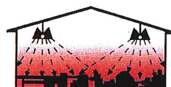
INFRARED HEAT Infrared heat works from the bottom up, warming people, floors, objects and machines first. Comfortable heat is retained in the lower working areas of your building.
