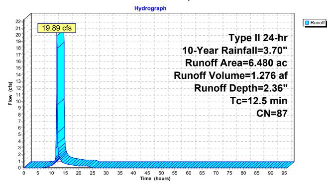
Prepared by Microsoft HydroCAD® 10.00-20 s/n 05053 © 2017 HydroCAD Software Solutions LLC
