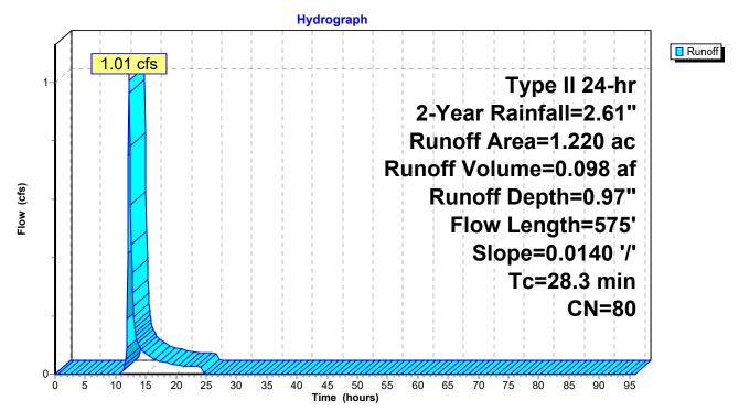
Prepared by Microsoft HydroCAD® 10.00-20 s/n 05053 © 2017 HydroCAD Software Solutions LLC
