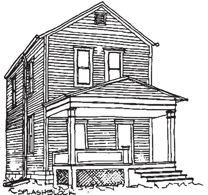
APPROPRIATE DOWNSPOUT LOCATION - ON SIDE FACADE
