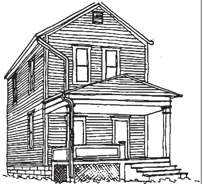
INAPPROPRIATE DOWNSPOUT LOCATION - OBSCURES ARCHITECTURAL FEATURES
