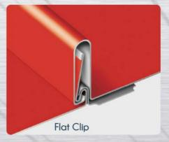
Clip at low point allows loads to be imposed on anchor clip, preventing rotation of seam and providing stronger interlock during an uplift event
