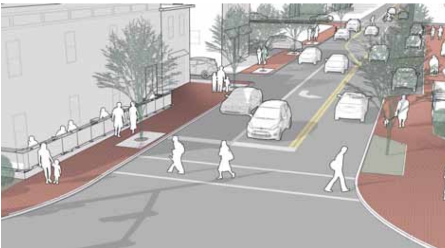
Adding a Separate Turn Lane
