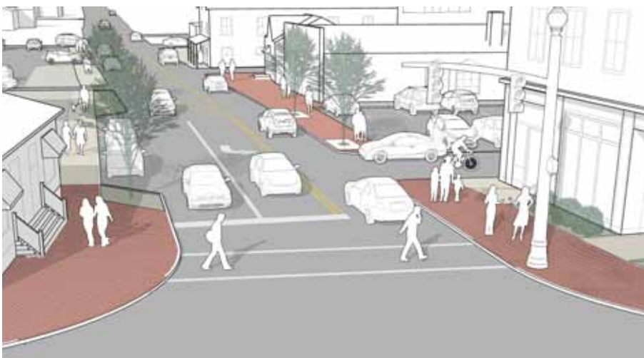
Adding a Separate Turn Lane
